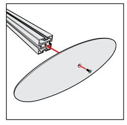
Base Plate & Extrusion Connection
