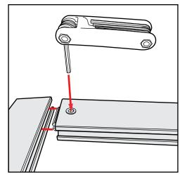
**Extrusion & Lock Connection**
