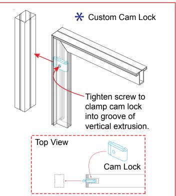
WHEN DISASSEMBLING ALUMINUM EXTRUSION, TIGHTEN ALL SETSCREWS AND LOCKS TO PREVENT LOSS DURING SHIPPING
