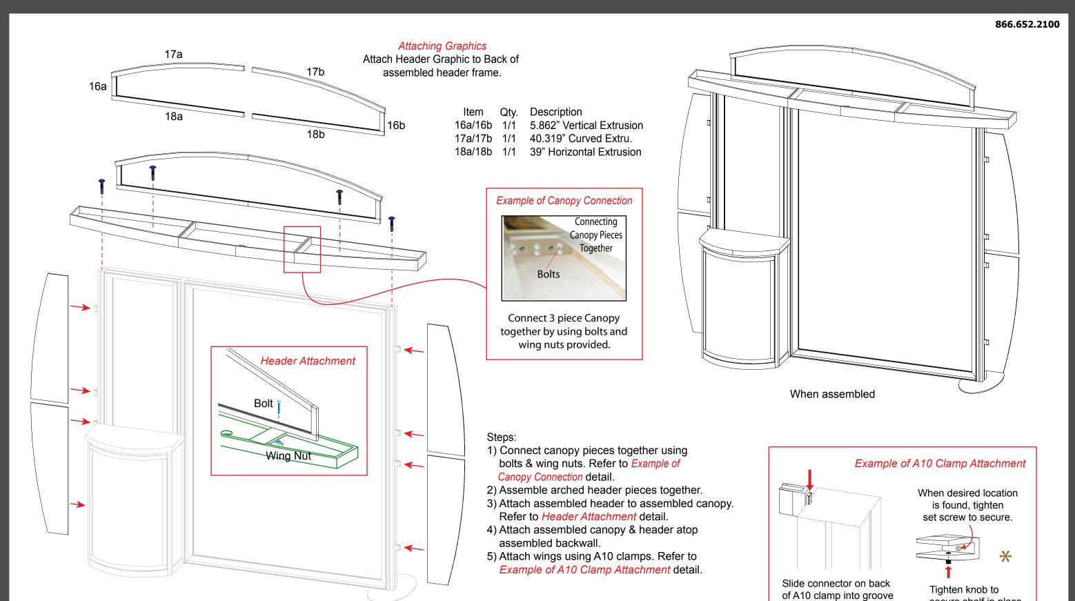
WHEN DISASSEMBLING ALUMINUM EXTRUSION, TIGHTEN ALL SETSCREWS AND LOCKS TO PREVENT LOSS DURING SHIPPING secure shelf in place.
